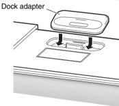
First align the front edge of the dock adapter, and then press down on the rear edge.
